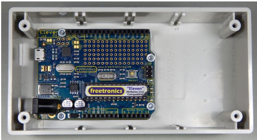
The Freetronics Eleven (Uno equivalent) board, mounted in the bottom of the case (see drilling template on pages 35 and 36).
